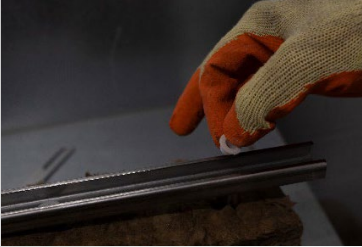
Figure 09 – Seating of nylon shoulder washers
