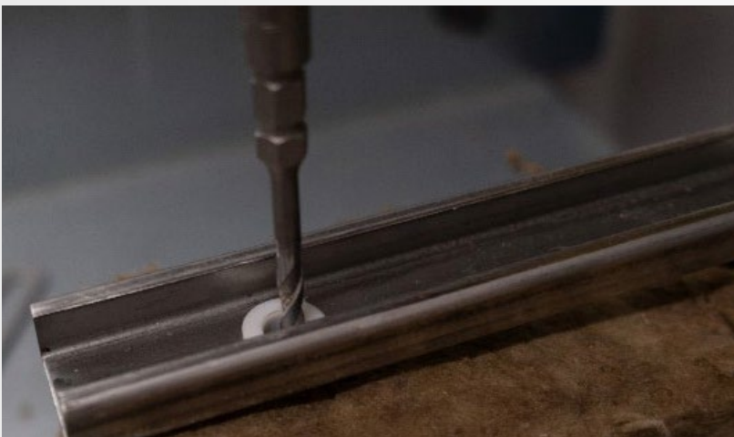
Figure11 – Drilling of pilot hole
