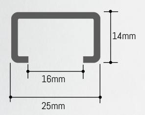
The 25/14 channel is available in 2700mm lengths and features closely spaced pre-punched holes to ensure a fixing position is always near the end, even when cut on-site. The channel has a 16mm opening to easily accommodate washers and fixings.
