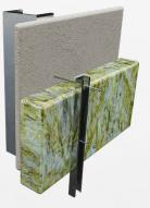
2. INSTALL FIXING THROUGH CHANNEL AND SLEEVE BACK TO INTERNAL STRUCTURE.
